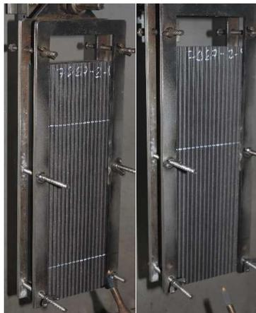
*Fig. 1. Ignitability test (flame application to surface and bottom edge).*
